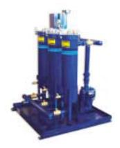
Triplex filters can be utilized for up to 5000 gallon tanks when uninterrupted flow is desired. Two vessels can filter while the third is being serviced. Also for interruptible service to 7500 gallons.
